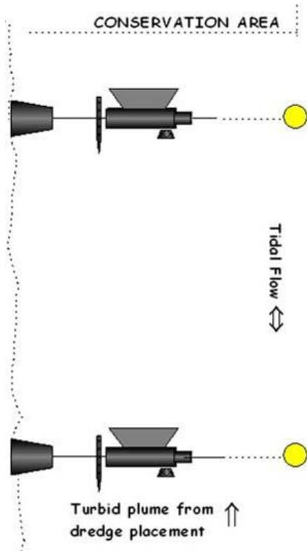
**Figure 2.** Combination nearfield-farfield sampling of suspended sediments (and tracer) using the time-series traps. This deployment/sampling strategy enables a wealth of information on the local sediment dynamics to be recorded, and for physical impacts to sensitive sites to be assessed with some confidence
