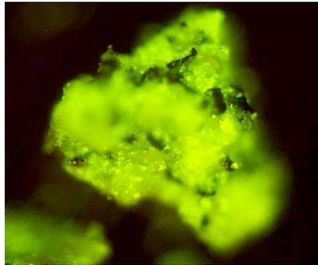
**Figure 1:** Partrac FM Series Tracer (scale: the particle is ~100  $\mu$ m in diameter)
